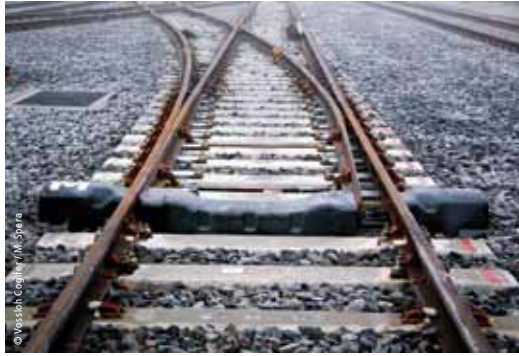
Easyswitch-R (open on the left, closed on the right), Lyon tramway line, Meyzieu station, France
